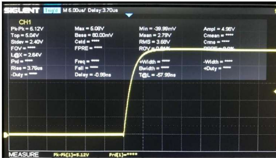
Figure 1 Optical pulse response (Typical Rise time).
