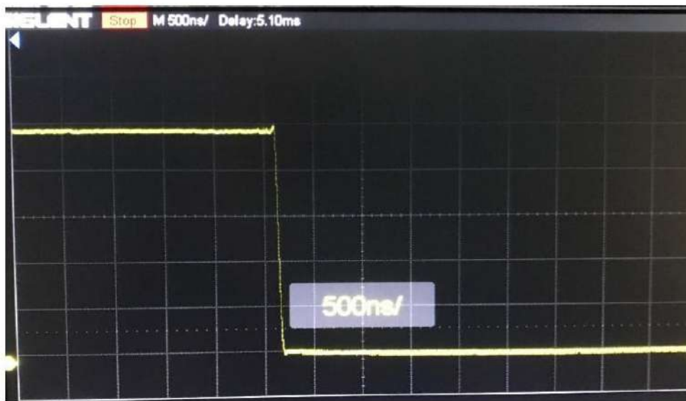
Figure 2 Optical pulse response (Typical Fall time).
